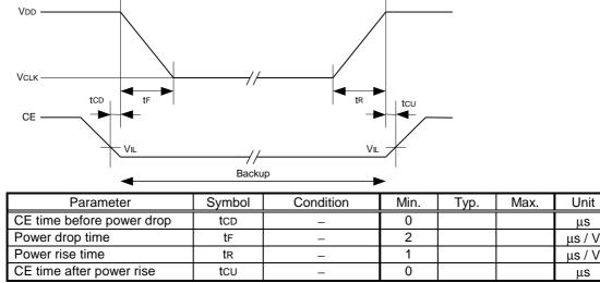
\* When main power souce input to VDD from backup condition, CE should be definitely LOW
