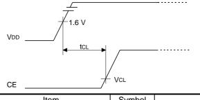
\* When the power is turned to ON, use with CE = "L" ( VcL[V] in the diagram ) as illustrated in the following timing chart.
