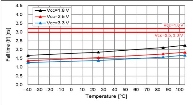
20% - 80% V<sub>CC</sub>, T<sub>use</sub> = +25 °C, 負荷(L<sub>CMOS</sub>)特性
