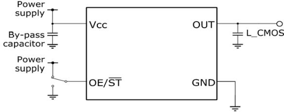
(2) #1 pin =  $\overline{OE}$ / $\overline{ST}$
