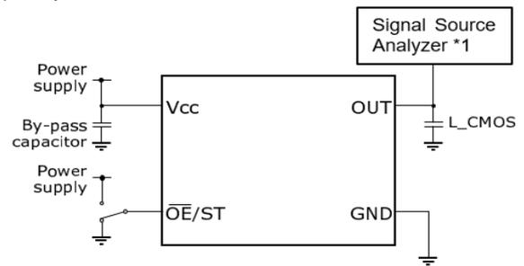
\*1 Signal Source Analyzer: Keysight: E5052B, Minimum frequency = 10 MHz
