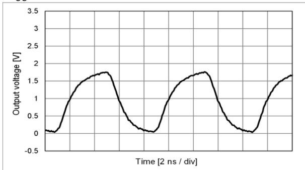
$f_o = 150 \text{ MHz}$ ,  $L_{\text{CMOS}} = 15 \text{ pF}$ ,  $T_{\text{use}} = +25 \text{ }^\circ\text{C}$ , tr/ff: A (標準) or B (最高速)
