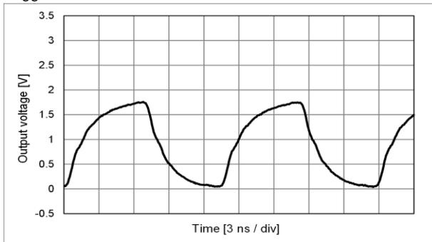
$f_o = 100 \text{ MHz}$ ,  $L_{\text{CMOS}} = 15 \text{ pF}$ ,  $T_{\text{use}} = +25 \text{ }^\circ\text{C}$ , tr/ff: A (標準) or C (高速)
