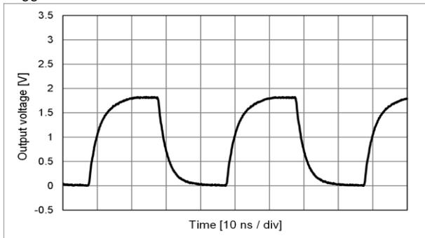
$f_o = 50 \text{ MHz}$ ,  $L_{\text{CMOS}} = 15 \text{ pF}$ ,  $T_{\text{use}} = +25 \text{ }^\circ\text{C}$ , tr/ff: A (標準) or E (最低速)
