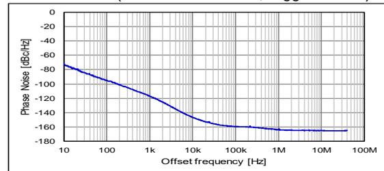
Phase Jitter (12 kHz to 20 MHz): 38 fs Typ.
