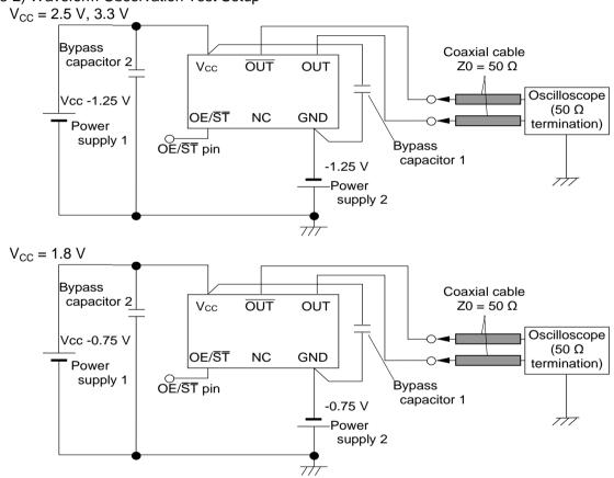
(8-2) Waveform Observation Test Setup
