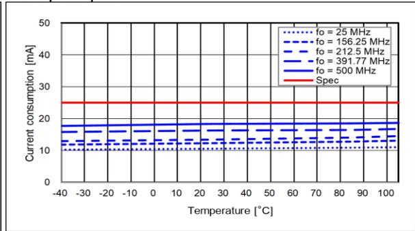
$V_{CC} = 2.5\text{ V}$ , Temperature Characteristic
