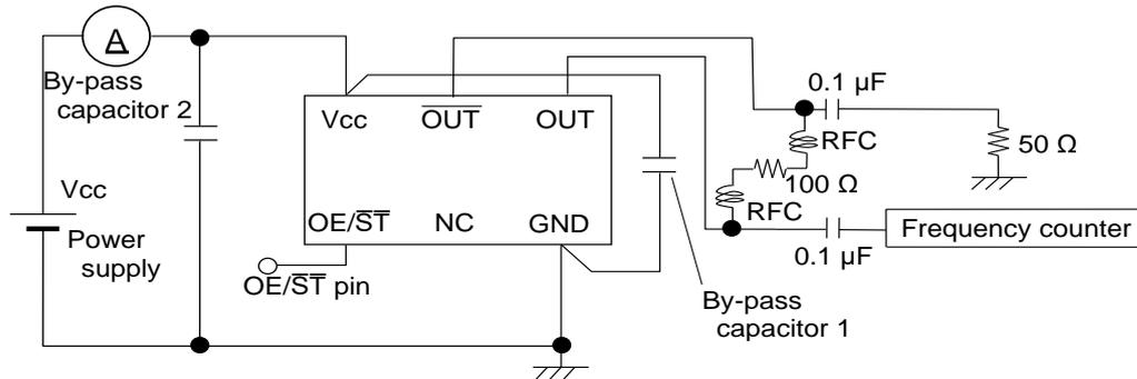
\* To measure Disable current or Stand-by current, OE/ST terminal is connected to GND
