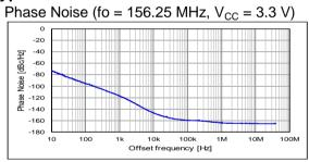
Phase Jitter (12 kHz to 20 MHz): 38 fs Typ.
