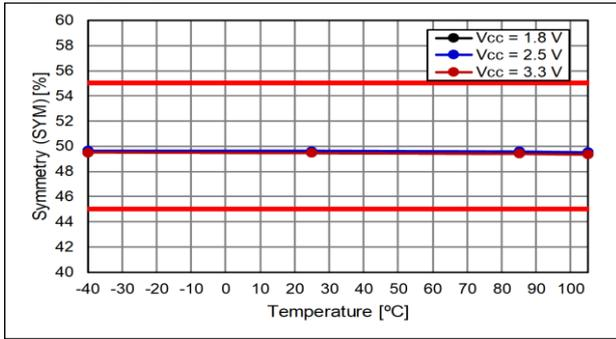
(7-5) Output Voltage Temperature Characteristic
