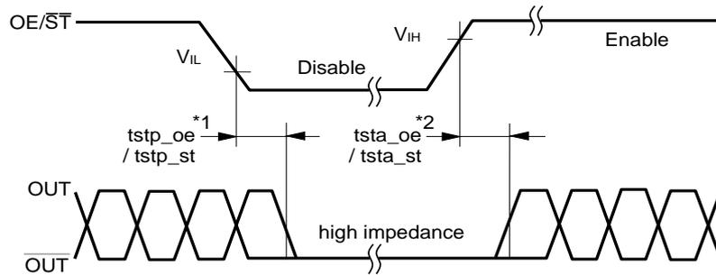
\*1 The period from OE/ $\overline{\text{ST}}$  =  $V_{IL}$  to OUT = High impedance (Disable)
