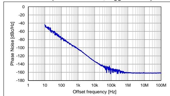
Phase Jitter (12 kHz to 20 MHz): 15 fs Typ.
