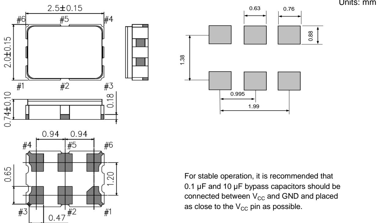
For stable operation, it is recommended that 0.1  $\mu$ F and 10  $\mu$ F bypass capacitors should be connected between  $V_{CC}$  and GND and placed as close to the  $V_{CC}$  pin as possible.
