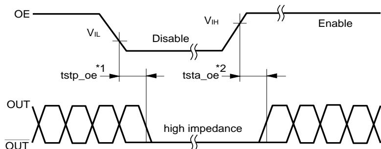
\*1 The period from  $OE = V_{IL}$  to  $OUT = \text{High impedance}$  (Disable)
