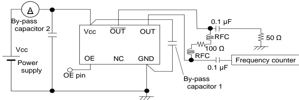
\* To measure Disable current, OE terminal is connected to GND
