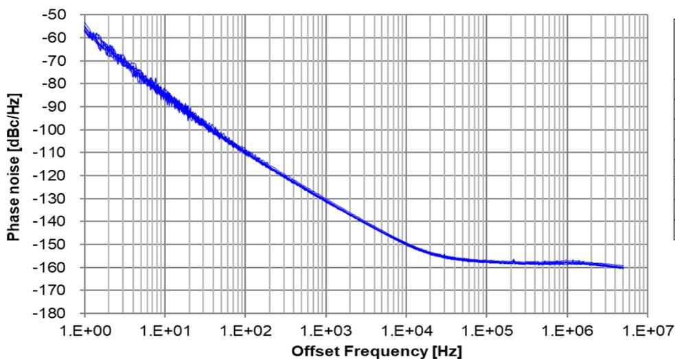
(4)  $f_o = 55 \text{ MHz}$ ,  $T_{\text{use}} = +25 \text{ }^\circ\text{C}$ ,  $n = 3 \text{ pcs}$
