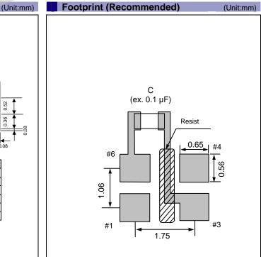
To maintain stable operation, provide a  $0.01 \mu$ F to  $0.1 \mu$ F by-pass capacitor at a location as near as possible to the power source terminal of the crystal product (between Vcc - GND).
