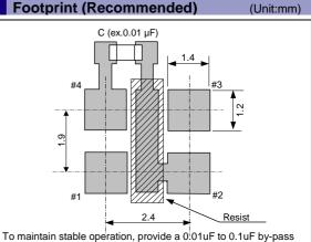
capacitor at a location as near as possible to the power source terminal of the crystal product (between Vcc - GND).
