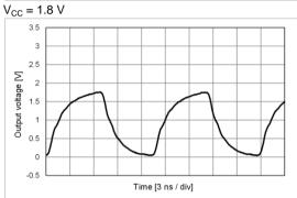
fo = 100 MHz, L\_CMOS = 15 pF, T\_use = +25 °C, Rise/Fall time: A (Default) or C (Fast)
