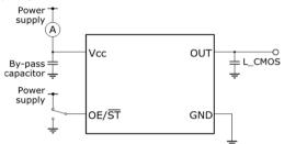
\* Disable current test should be OE = GND. Stand-by current test should be  $\overline{ST} = GND$ .
