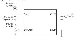
\* Disable current test should be  $\overline{OE} = V_{CC}$ . Stand-by current test should be ST =  $V_{CC}$ .
