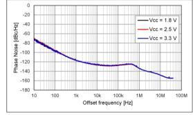
Phase jitter: 1.2 ps Typ. Offset frequency: 12 kHz to 5 MHz
