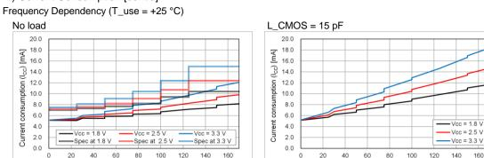
The actual current consumption is the total of the current under the condition of no load and the current to drive the output load (fo x L\_CMOS x  $V_{CC}$ ). To reduce the current consumption, it is effective to use lower frequency, lower supply voltage and lower output load.
