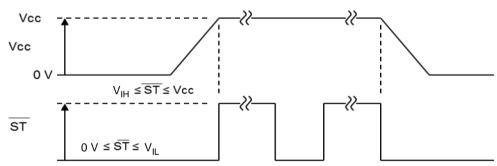
When standby control and  $V_{\text{CC}}$  control are the same
