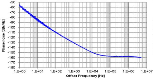
Offset Phase Freq. noise [dBc/Hz] [Hz] -56 1 Hz 10 Hz -85 100 Hz -110 1 kHz -131 10 kHz -150 100 kHz -157 1 MHz -158 5 MHz -160
