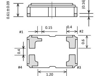
Terminal coating: Au plating Reference weight Typ.: 8.1 mg
